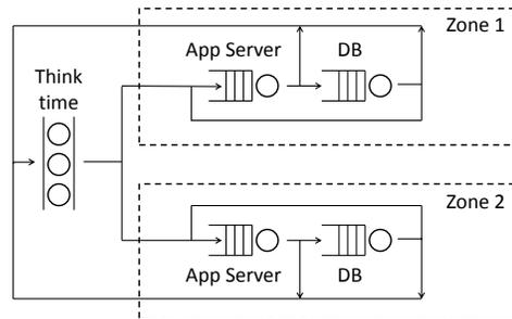
Fig. 7. Model of the 2-zone deployment
