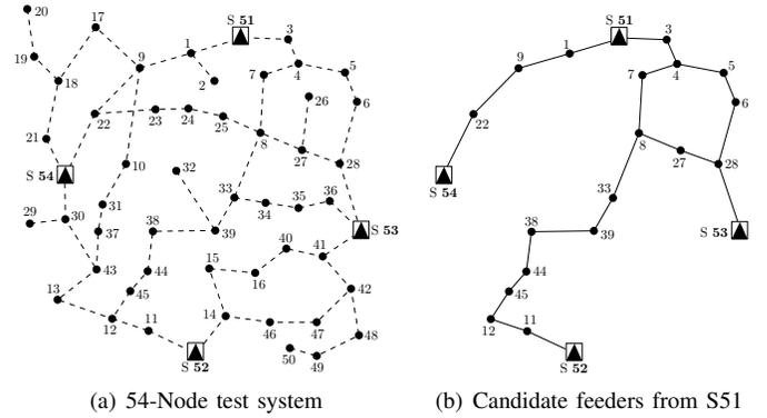
Fig. 4. Candidate feeders by minimum cost flow method.
