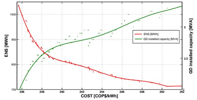
Fig. 4. GD installed capacity vs ENS
